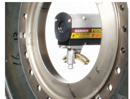
Measuring Residual Stress inside a Bore
