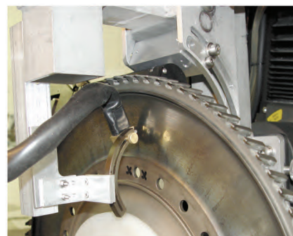
Measuring Residual Stress Inside A Bolthole
