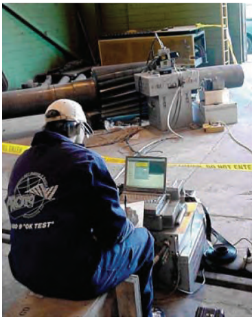
Fig. 7: Measuring residual stress on a component in the field
