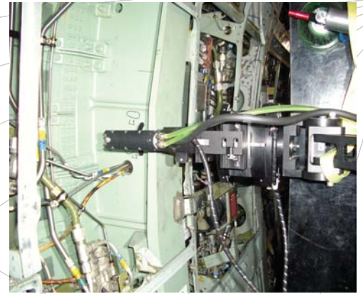
Measuring Residual Stress on an Airframe with an iXRD Portable System
