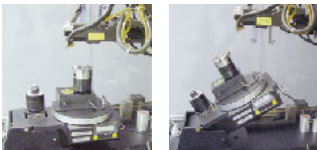
Automated orientation fixture for programmed sequence measurement
