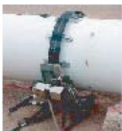
No. 1 Field Stand Pipeline or pressure vessel-capable with magnetic flex track and manual X,Y axis, auto Z axis (Suction cup foot option available for all stands)
