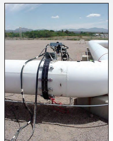
MEASURING RESIDUAL STRESS ON A PIPELINE
