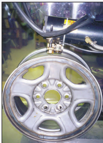
MEASURING RESIDUAL STRESS ON A WHEEL
