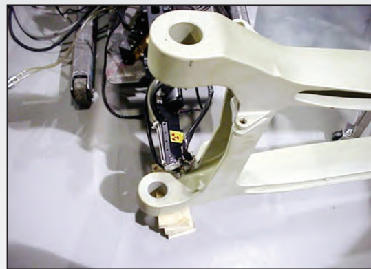
MEASURING RESIDUAL STRESS ON A LANDING GEAR
